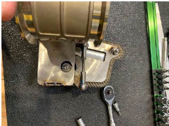
Step 22. Attach the OE adjustable control arm ball sockets to the ball ends of the MF control arm and valve assembly.
