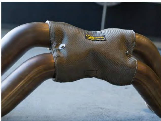
Step 26. The X-Pipe Assembly comes with a Heat Blanket installed as shown.
