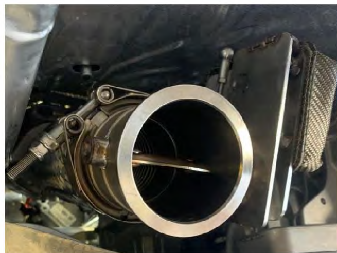
Step 24. Attach both valve assemblies to the installed Inlet Pipe Assemblies using the supplied clamps.
