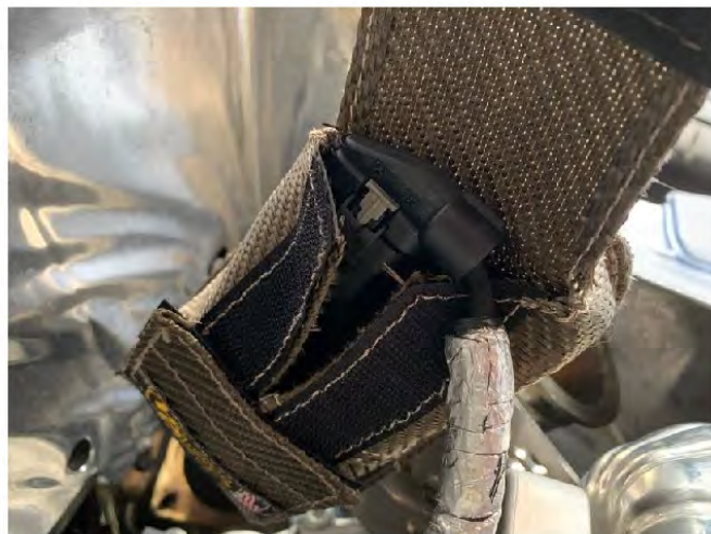
Step 25. Reconnect both electrical connectors to the valve motors. Close the Heat Blanket.
