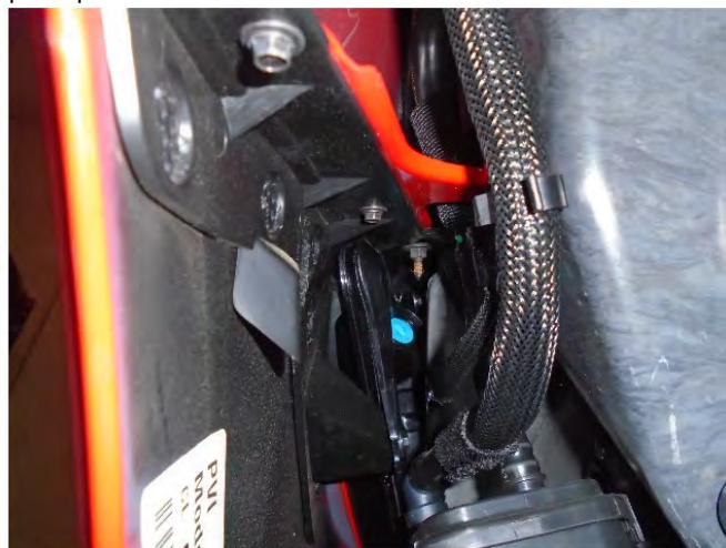
Step 8. The bumper and rear valance must be removed together. First remove the 10mm nut attached to the smog pump on the passengers side of the vehicle.
