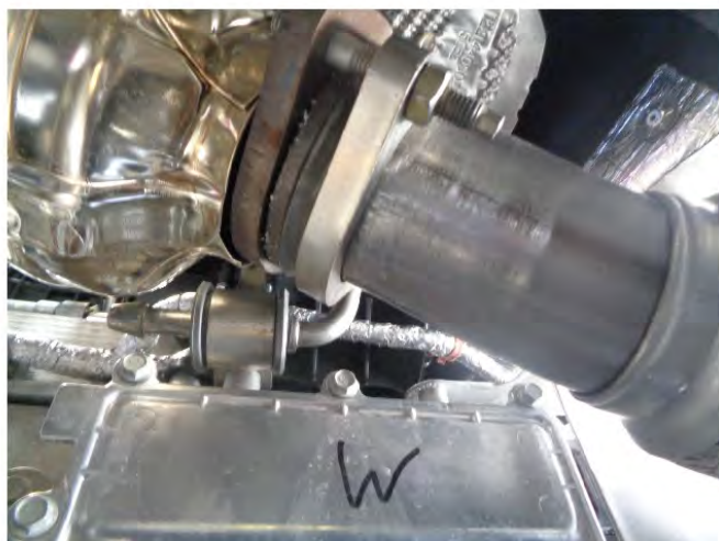
Step 23. Loosely attach both Inlet Pipe Assemblies to the vehicles catalytic converter outlets (D/S shown).
