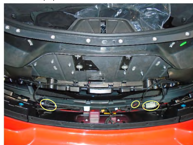
Step 11. Disconnect the three harness plugs for the rear lights. The rear bumper and valance can now be removed.
