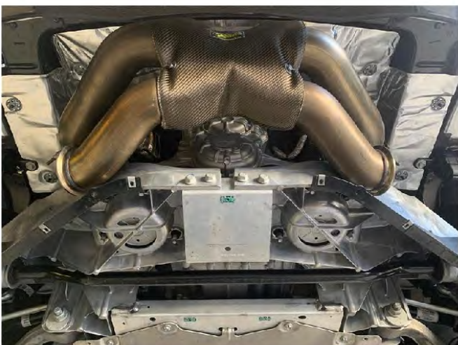
Step 27. Loosely attach the X-Pipe Assembly to the valves you just installed using the supplied clamps.
