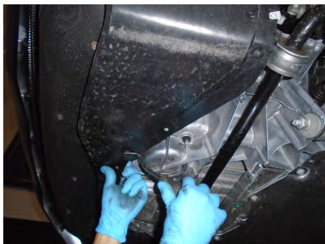
Step 7. Remove the secondary covering attached to the rear valance by removing (4) T-15 Torx head screws and (2) push pin clips..
